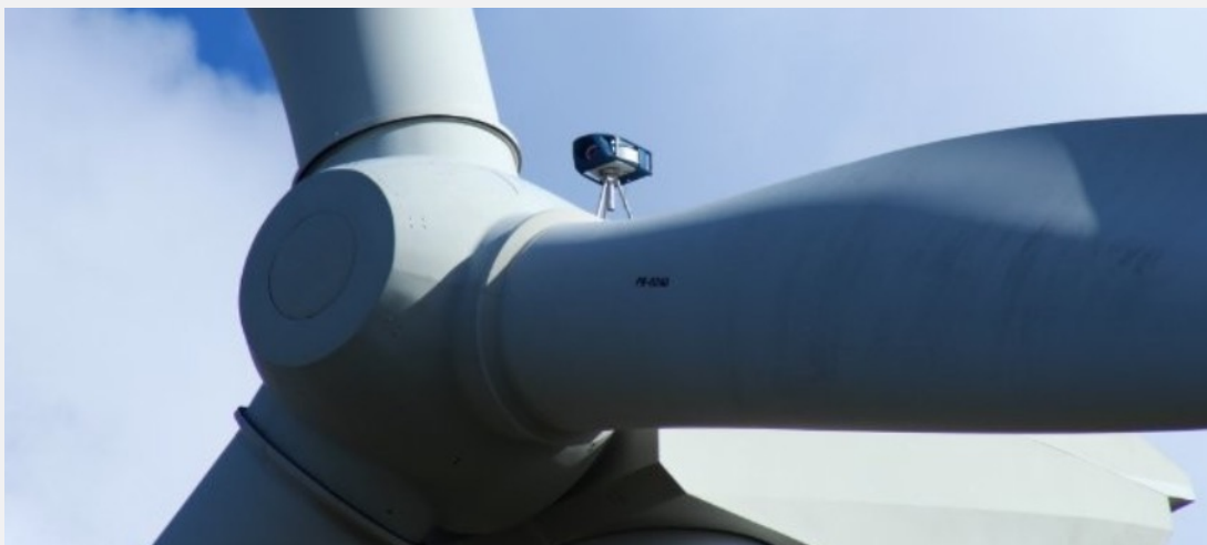
Figure 4 – Horizontal LIDAR is being deployed by NTR to detect static yaw misalignment
